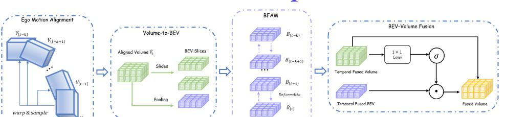
Our temporal fusion module enhanced the scene representation through ego-motion alignment in voxel space and a Backward-Forward Attention Module (BFAM) in BEV space.
